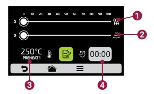
**c)** To change the speed of hot air and microwaves, simply drag your finger over the bar of each parameter or click on the desired location in the bar.
